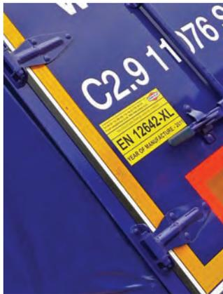
**Certified:** XL-rated vehicles are manufactured to a higher standard than normal trailers
