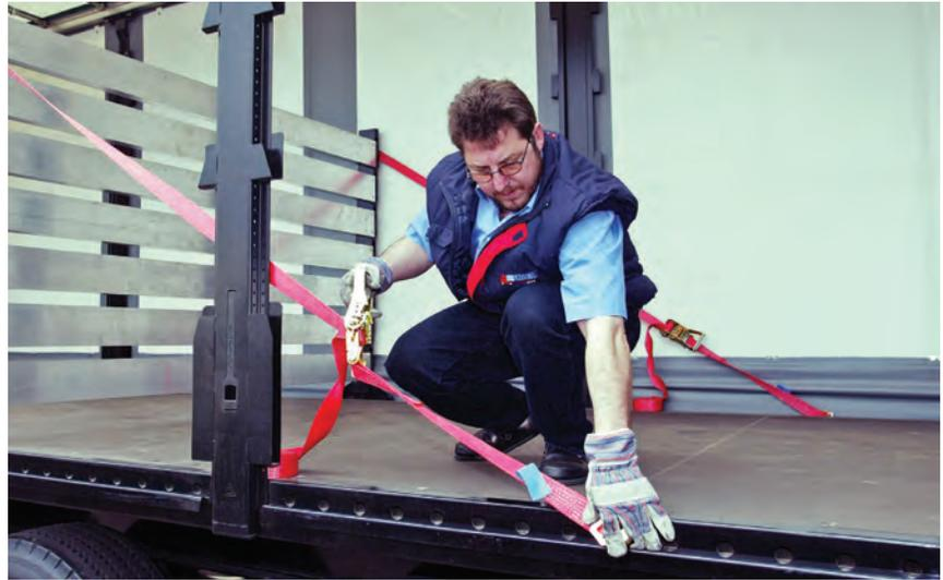
**Positive fit:** Unless the load is a positive fit operators will still need to strap it up
