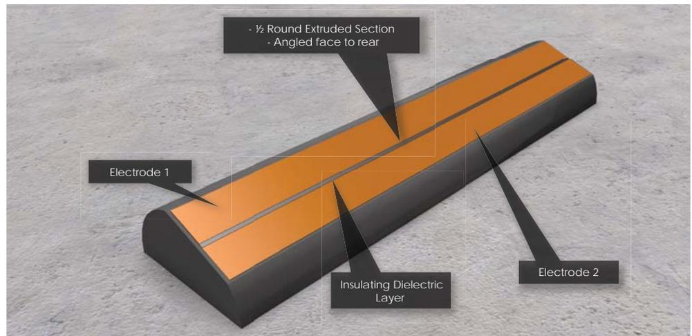
The amount of power required to run Plasma Actuators is extremely low (circa 30W dependent on length) and thus could be powered by a simple trickle charged battery or even a small solar panel fitted to the roof of the vehicle.
