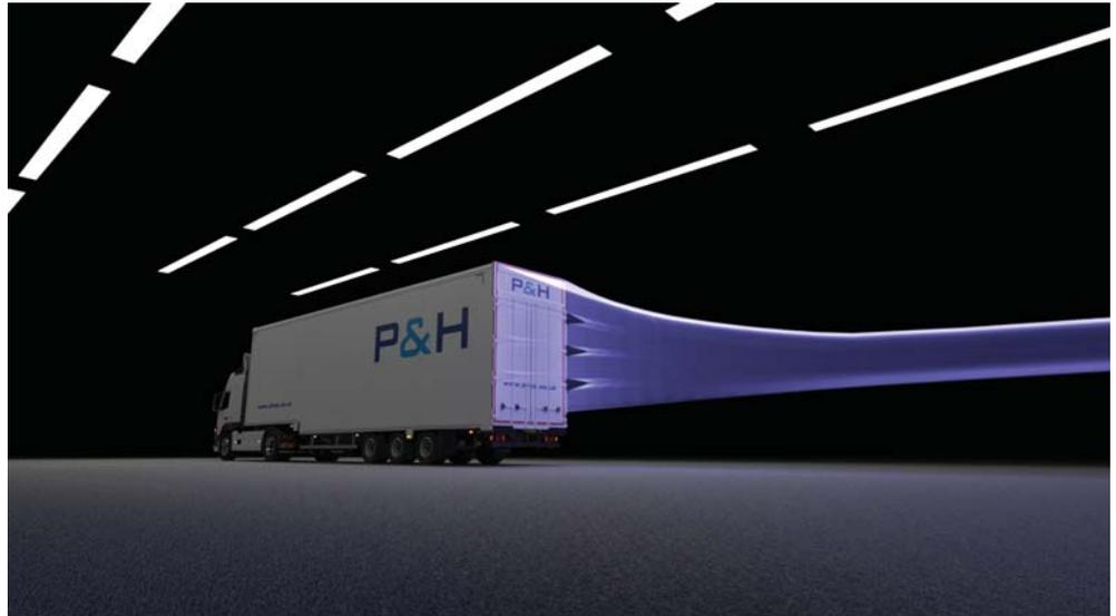
Studies on standard physical boat tails have found that up to 7% in fuel reduction can be achieved and plasma actuators are expected to generate similar fuel savings. However, many operators are unwilling to invest in standard physical boat tails due to the high risks of damage and associated costs to repair.
