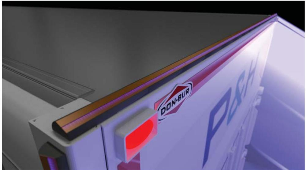
The Plasma Actuators are positioned at the end of the trailer along the sides and top of the rear frame and are angled inwards and downwards, respectively. Once activated, the resulting airflow is up to 10 m/s, then to avoid any discomfort to pedestrians, they are deactivated by a speed sensor once the vehicle reaches less than 10mph.
